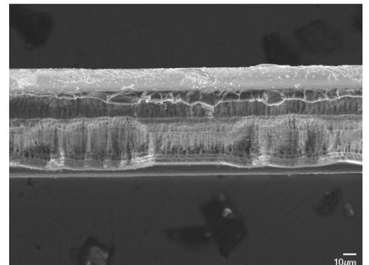
Side-view of the bioresorbable fiber Bragg grating immersed in physiological solution for up to 56 h.
